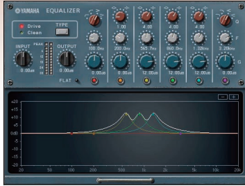
Figure 8. Graphical user interface panel of the “Equalizer 601”
