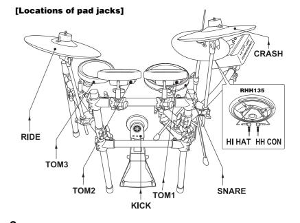
3. In the case of snare and tom pads, wrap the cables around the cable clips to prevent them from being pulled out.
