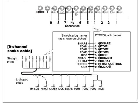
2. Plug the 9-channel snake cable's L-shaped plugs into the correct pads.
