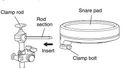
3. If necessary, use clamp bolts A to E to adjust the height and angle of the snare pad. When doing so, be sure to adjust one bolt at a time (i.e., loosen a bolt, adjust the pad, and then retighten before loosening another).
