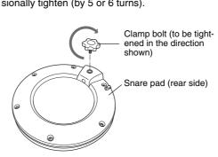
**2.** Mount the snare pad on the rack's clamp rod. As shown below, ensure that the rod section is fully inserted into the pad's mounting hole, and then fully tighten the clamp bolt
