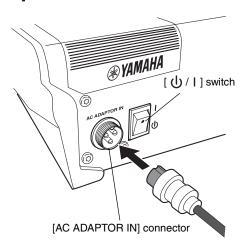
② Turn the fastening ring clockwise to secure the connection.
