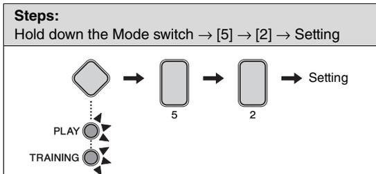
The term “crosstalk” refers to the output of spurious trigger signals from a pad other than the one that was struck as a result of vibration or interference between pads. You can adjust the Crosstalk parameter for individual pads to prevent this phenomenon from occurring.
