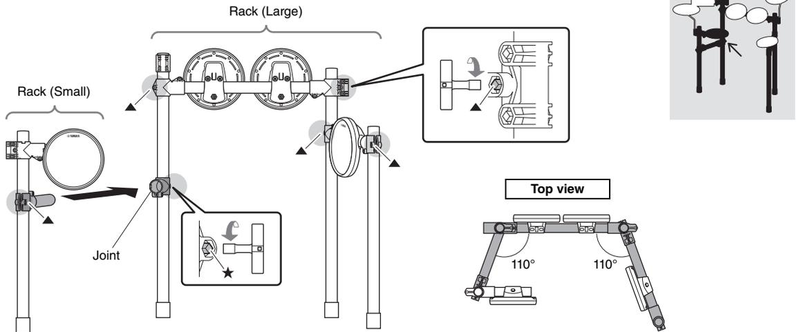
1. Loosen the ★ key bolt on the rack (Large) and turn the joint around before sliding the Small rack (in the next step).
