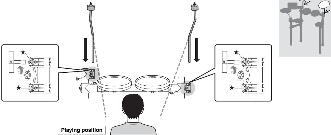
1. Loosen the four ★ key bolts at the ends of the tom 1/2 part.
