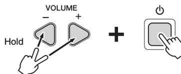
The drum module's lights will flash and the Factory Reset will be restored.
