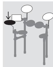
1. Loosen the ★ key bolt on the stopper, which is located at the top of the hi-hat holder.
