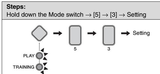
You can specify the type of snare pad connected to your drum module.
