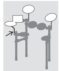
1. Loosen the two ★ key bolts in the back of the snare part.
