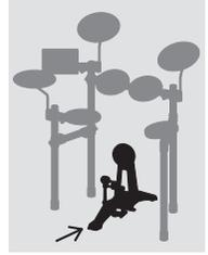
1. Remove the four wing bolts, spring washers, and flat washers from the kick pad, and arrange each set nearby in the disassembled condition.
