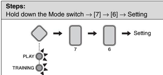
You can set the [PHONES/OUTPUT] jack to output either mono or stereo sound. We recommend that you select the Mono setting if connecting a standard mono-audio cable to this jack in order to use your drum module with external speakers, a mixer, or other similar equipment.
