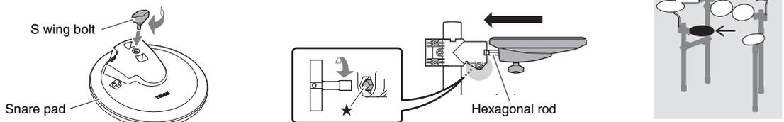
1. Take the snare pad and the S wing bolt and lightly tighten the S wing bolt. (Five or six turns is sufficient.)
