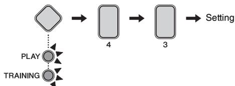
You can adjust the position at which the hi-hat switches from open to closed when you operate the hi-hat controller. The lower the value, the smaller the virtual opening between the top and bottom hi-hats. Larger values increase the size of the gap between the top and bottom cymbals, and this can prevent foot close or foot splash sounds from being produced when you operate the pedal.
