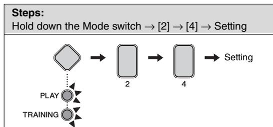
You can easily configure the drum module to produce a kick drum sound when you operate the pedal connected to the **[HI-HAT CONTROL]** trigger input jack. This convenient function provides support for double bass drumming techniques.
