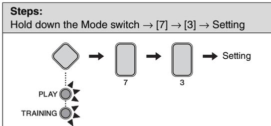
You can set whether the USB audio input is sent to the USB out or not. When set to “Output,” the audio data input from a PC (for example) is mixed with your pad performance and they are sent together to the USB out. When set to “Not out-put,” only your pad performance is sent to the USB out, even if the audio data is input and played from the PC.
