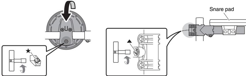
1. Loosen the ★ key bolt on each of the pads.
