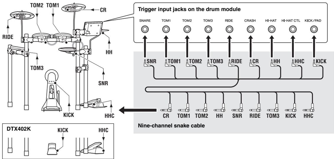
1. Insert the mini plugs\* at one end of the nine-channel snake cable into the correct trigger input jacks (SNARE to KICK/PAD) on the drum module. (\*: The smaller set of plugs.)
