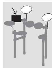
1. Loosen the ★ key bolt on the back left of the rack and turn the joint around before sliding the sliding the drum module (in the next step).
