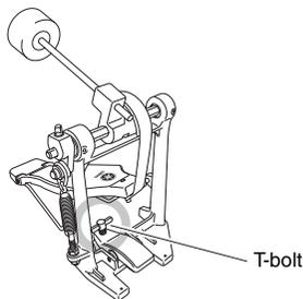
6. Fit the raised section at the front of the kick pad holder into the foot-pedal's assembly bracket.
