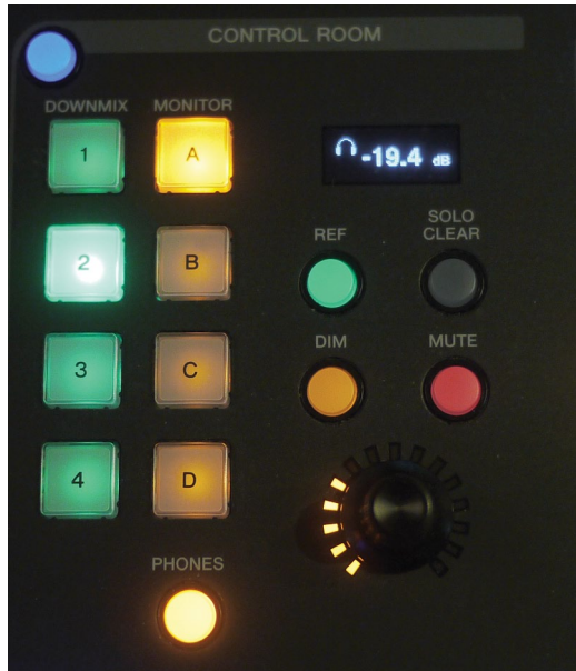
Figure 7.18 Control Room OLED display in Phones mode
