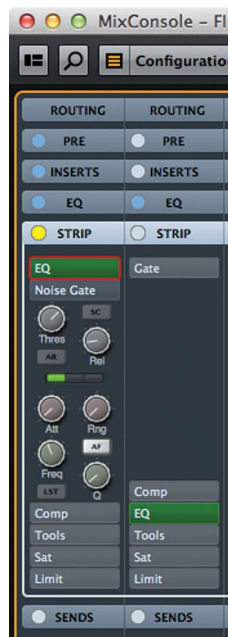
Figure 6.73 EQ Tab moved to the first position in the channel's signal flow
