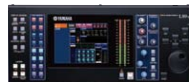
Press one of the 16 MIX/MATRIX keys twice and all other MIX/MATRIX keys will light while the pressed button flashes. At the same time "SENDS ON FADER" will flash on the display to indicate that the Sends On fader mode is active.
