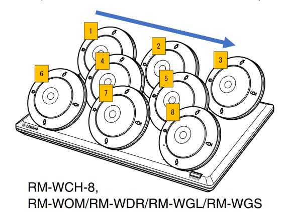
2. Wait for the firmware update of the last placed microphone to complete. After confirming the completion of the last microphone firmware update, return to 1) and perform the next firmware update.
