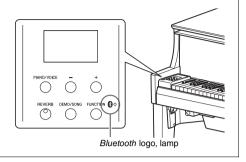
• *Bluetooth* is a technology for wireless communication between devices within an area of about 10 meters (33 ft.) employing the 2.4 GHz frequency band.
