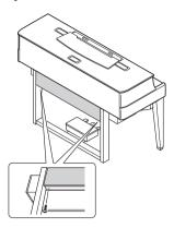
7 Insert the AC power cord plug into the [AC IN] connector.
