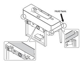
3-2 Move the main unit slightly toward the rear side, then adjust its position so that the projecting pin on the metal brackets on the bottom of the main unit will lock into the notch on the metal brackets of the legs (L/R).
