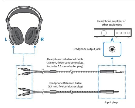
Firmly plug the balanced or unbalanced cable into the headphone output jack on the device to which you want to connect.
